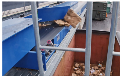
A chute leads the briquettes to a container outdoors.
