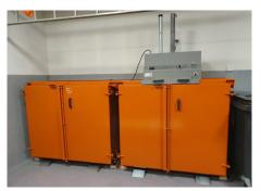
Quality Hotel Ramsalt in Bodø, chose the Orwak multi-chamber baler 5070-Combi, which reduces the amount of residual waste by up to 70 %. This is of great importance for any business focusing on operating costs and on cutting  $CO_2$  emissions. EnviroPac recommended and delivered this multi-chamber solution. The baler is top-loaded meaning that the chambers are open and it is easy to throw waste straight into the two 4-wheel plastic 660 L bins, which are placed in the baler.
